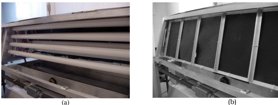
Figure 1. UV Exposure: (a) lamps details (b) geomembranes samples exposed to UV radiation
