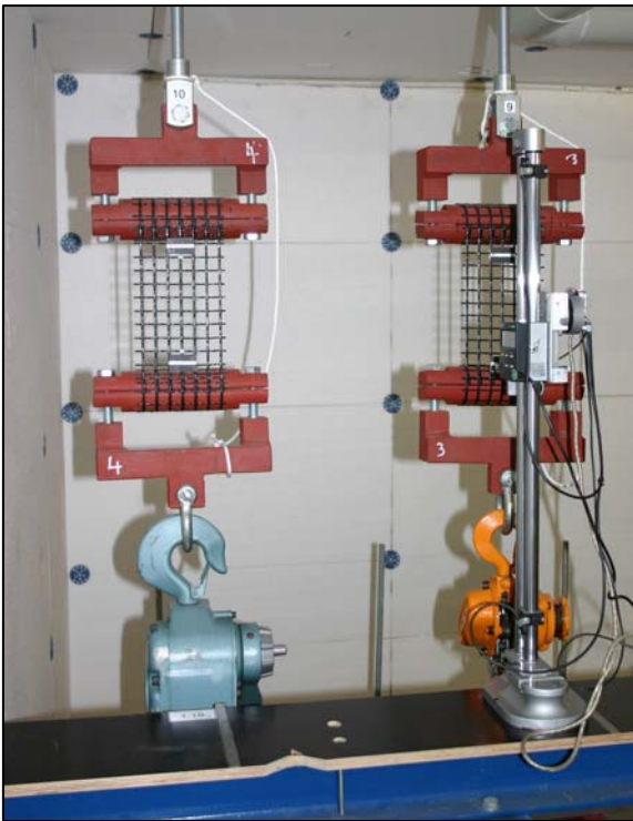
Figure 3. Specimens with deformation measurement system
