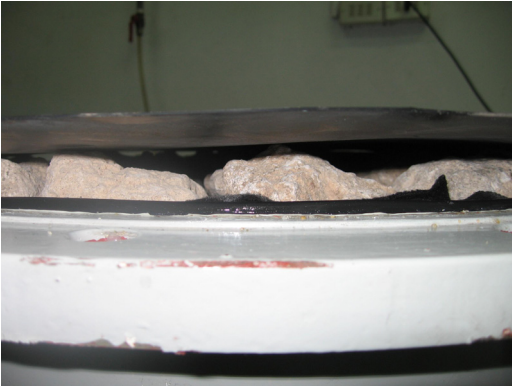
Figure 2. The liner is placed over the test area.
