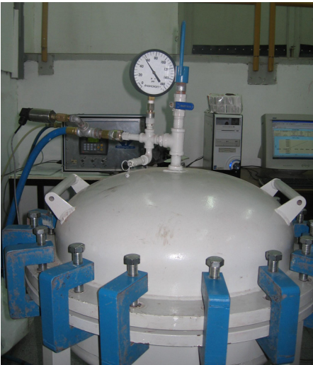
Figure 3. The pressure dome is installed over the liner and slowly pressure is increase until 100 psi during 24 hours.
