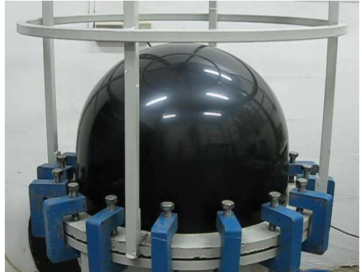
Figure 5. The multi-axial deformation in a LLDPE geomembrane, smooth or textured (see figure 6) easily exceeds the GM17 standard >30%
