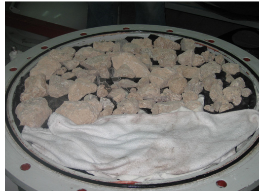
Figure 1. The test area (60 cm diameter) was divided in two sectors. One with geotextile and the other with coarse gravel.
