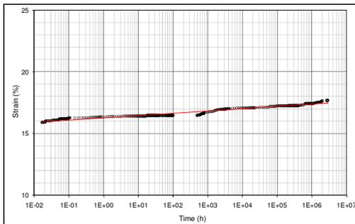
Figure 4. Creep master curve obtained from confined-accelerated creep test at 20% of the geotextile ultimate tensile strength in cross-machine direction.
