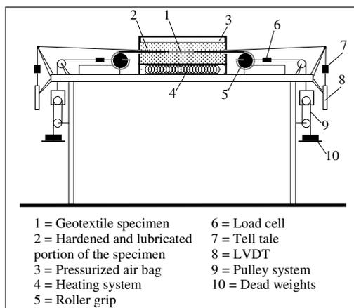
Figure 1. Layout of the machine developed in this research.
