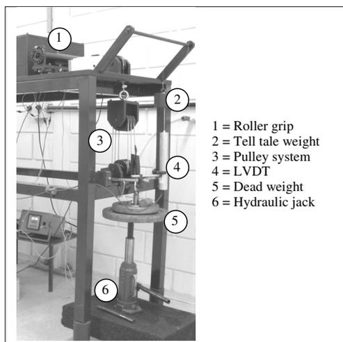
Figure 2. Lateral view of the machine developed in this research.
