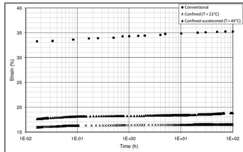
Figure 3. Conventional creep test result at 20% of the geotextile ultimate tensile strength in cross-machine direction.
