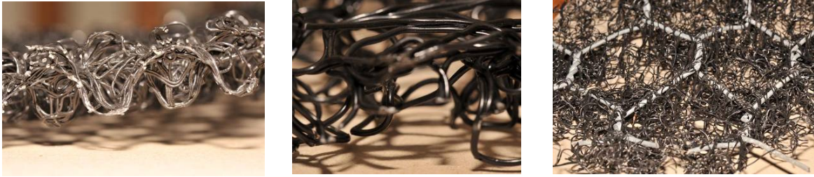
Figure 1...3: Claw mats of polypropylene as mazy laid structure and in combination with a grid net
