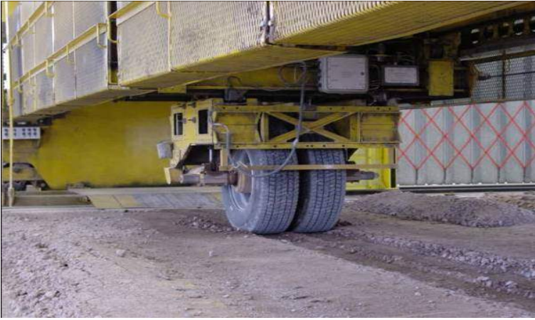
Figure 2(a). Full scale trafficking testing for an empirical model
