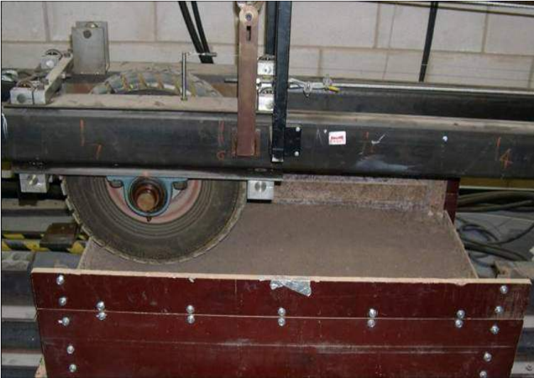
Figure 5. University of Nottingham slab testing equipment
