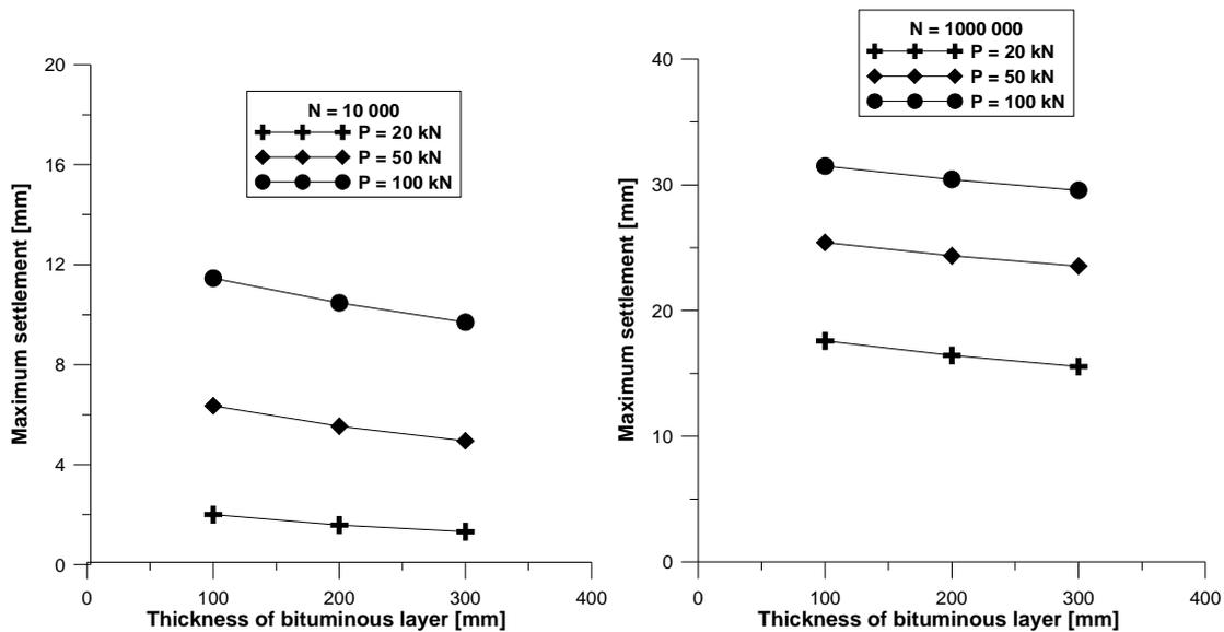
Figure 8. Influence of bituminous thickness on maximum pavement settlement.
