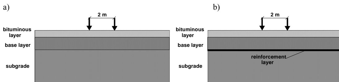
**Figure 1.** Schematic representation of structures used in analyses: a) pavement without geosynthetic; b) pavement after inclusion of the geosynthetic layer.
