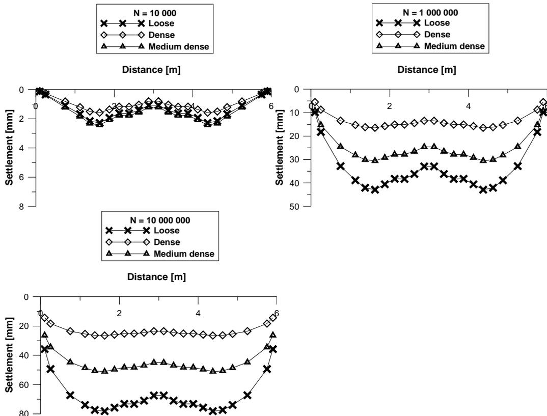
**Figure 3.** Surface settlement profiles for various initial densities of subgrade sand. Magnitude of loading:  $P=20\text{kN}$ .
