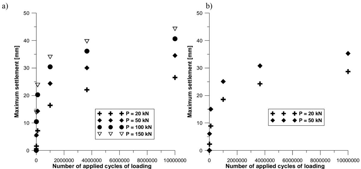
Figure 10. Influence of number of load application on maximum settlements: unreinforced (a) and reinforced (b) pavement.
