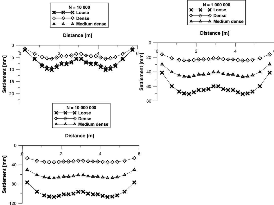
Figure 4. Surface settlement profiles for various initial densities of subgrade sand. Magnitude of loading: P=50kN.
