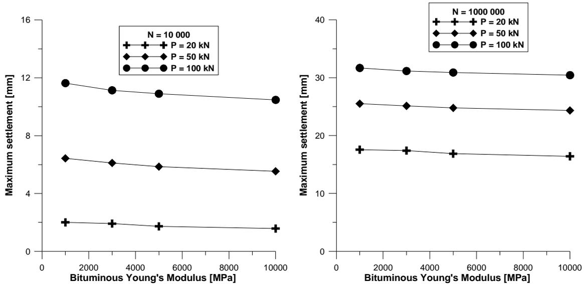
Figure 9. Effect of changing bituminous layer Young's Modulus on maximum pavement settlement.
