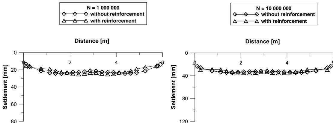
Figure 5. Comparison of reinforced and unreinforced pavements settlements. Dense sand used as subgrade.
