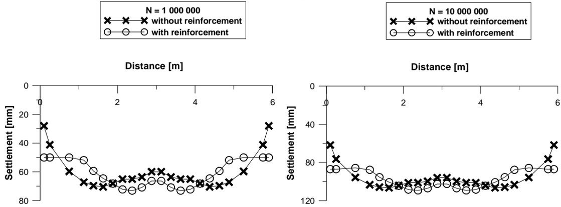
Figure 6. Comparison of reinforced and unreinforced pavements settlements. Loose sand used as subgrade.
