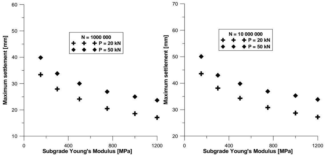
Figure 7. Effect of changing subgrade Young's Modulus on maximum pavement settlements. Pavement with geosynthetic layer.
