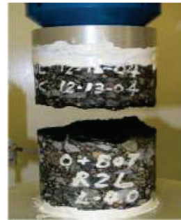
Figure 6. Adhesion tests show paving fabrics improve bonding between layers.
