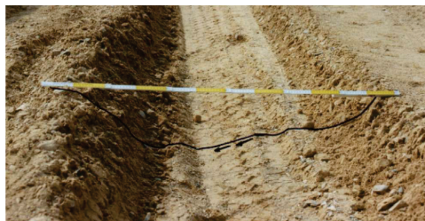
Figure 3. Rutting on a construction site.
