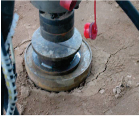
Figure 7. Cracks at the sub base surface.
