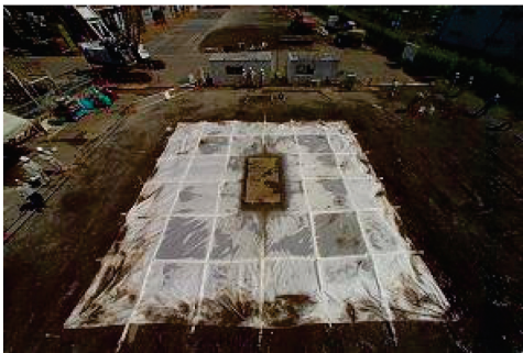
Photo 1. Panoramic view of the loading test for the LFR sheet.
