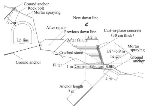
Figure 3. Determined remedial plan.
