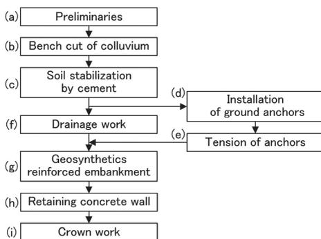
Figure 5. Construction flow.
