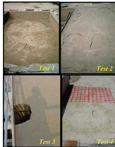
Figure 3. Surface settlement in Test 1 to Test 4.
