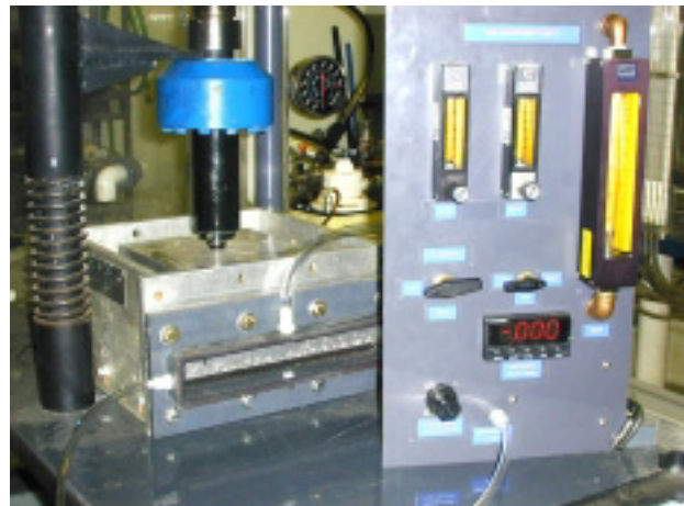
Figure 2. Photo shows the set up used for measuring gas transmissivity
