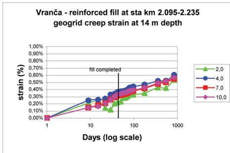
Figure 4. Vranča, geogrid creep strain vs. time.
