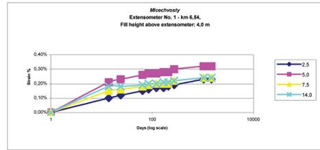
Figure 2. Mlcechvosty, creep strain of polyester strips.
