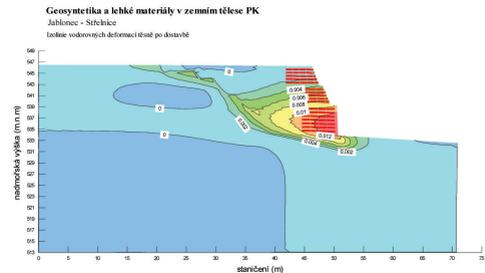
Figure 5. Jablonec, calculated horizontal deformations of the reinforced fill structure.
