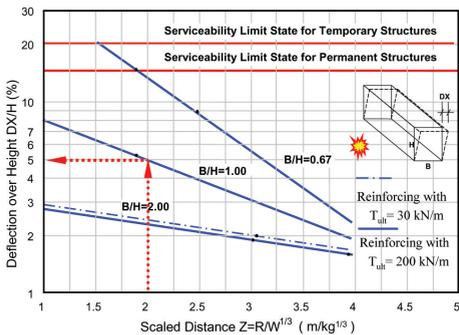
Figure 6. The design chart for RS walls.
