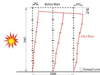
Figure 3. Deformed shape of RS2 (Blast Trial 2004).
