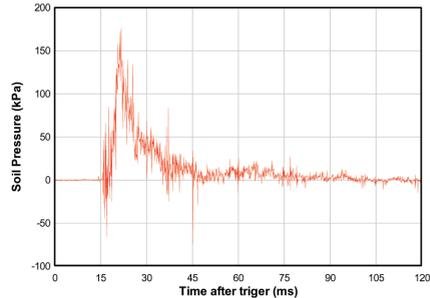
Figure 5. Typical soil pressure (Blast Trial 2004).
