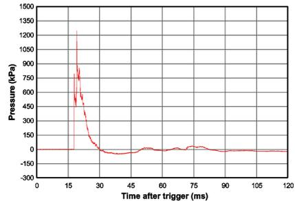
Figure 4. Typical blast air pressure (Blast Trial 2004).
