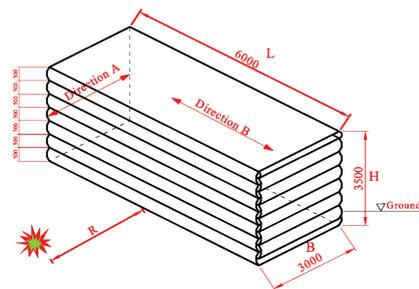
Figure 1. Typical configuration for RS wall.
