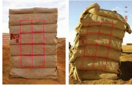
Figure 2. RS2 before and after 6 ton blast (Blast Trial 2004).
