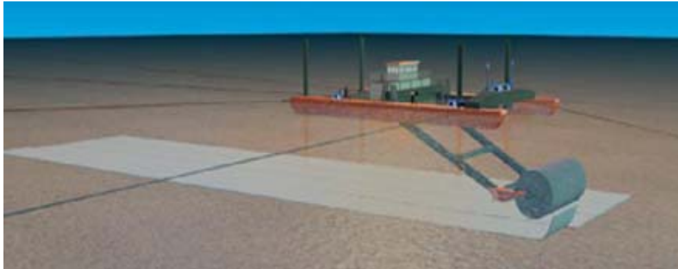
Figure 8: The BFM unrolling operation
