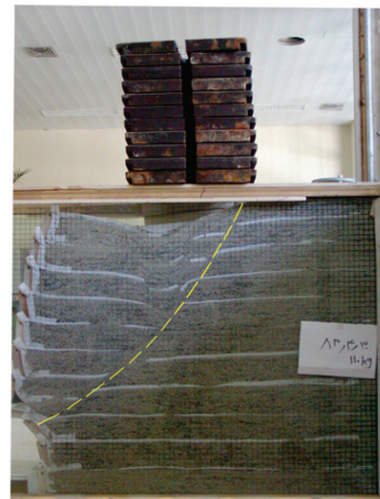
Photo 1. Failure of reinforced soil wall under the external surface load.
