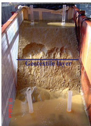
Figure 7. Local failure model 5.
