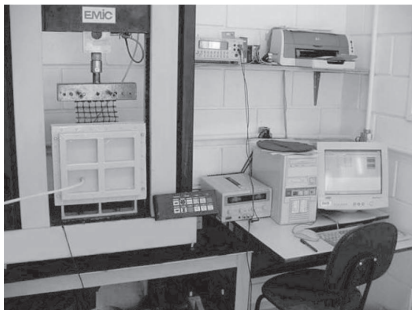
Figure 1. Device for small-scale tests.
