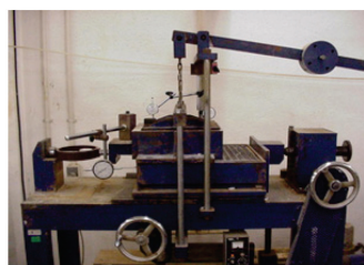
Photograph 1. The large-scale shear box test apparatus.
