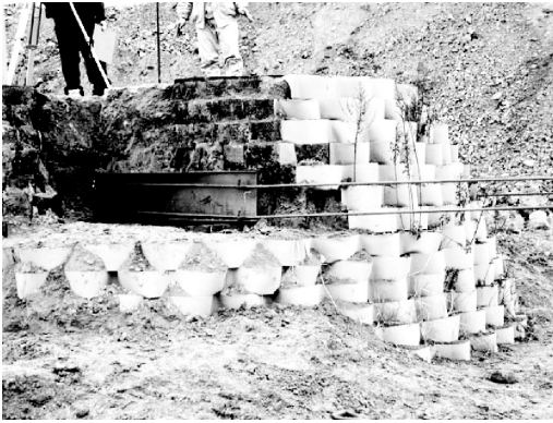
(a) Preparation of failure test
