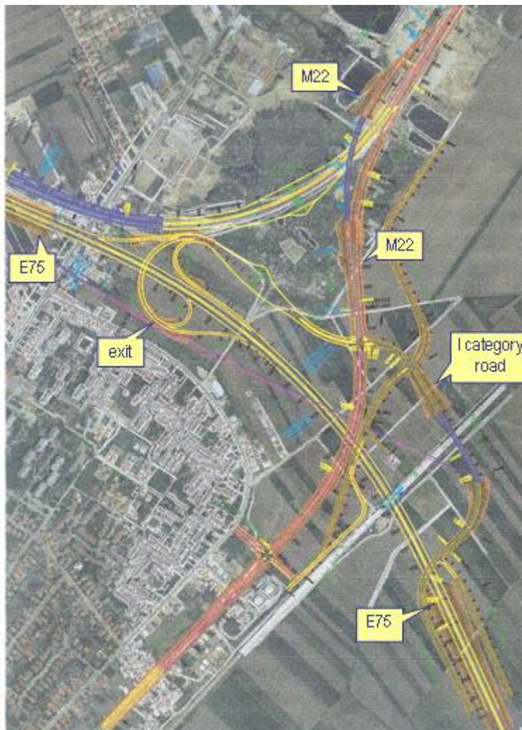
Figure 1. Aerial photo of "Batajnica" interchange with all road routes and indicated light-weight structures made of EPS blocks
