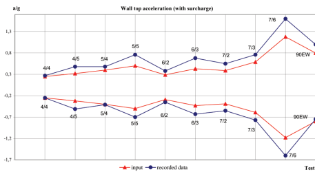
Figure 12. Acceleration amplification values at the top of the wall for the test with surcharge.
