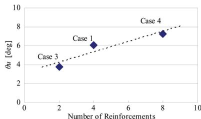
Figure 5. Relationship between the number of reinforcements and the gradient collapse angle.
