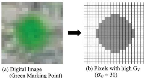
Figure 3. Extract pixels of marking point.
