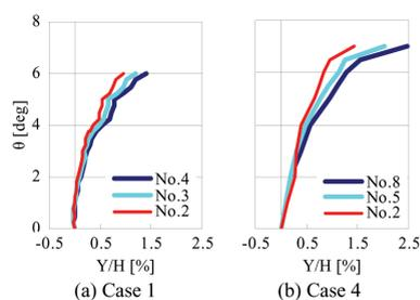
Figure 6. Horizontal displacement of walls.
