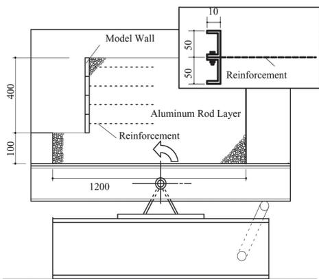
Figure 4. Experimental device.
