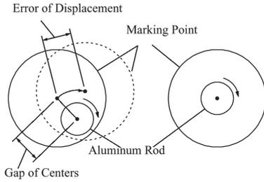
Figure 2. Error of displacement by rotation of aluminum rod.
