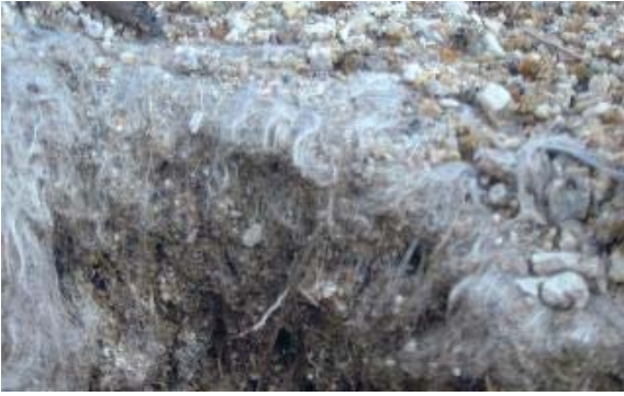
Figure 13. Anti-erosion effect of fibres in the SM025F6d section
