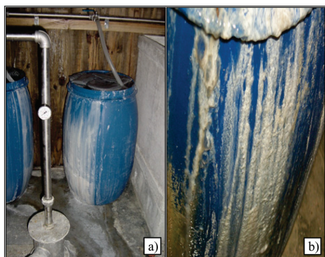
Figure 1. (a) Geosynthetics in vats with running sulphurous water, near the collecting zone in Unhais da Serra Medical SPA. (b) A close detail of the white residue referred in (a); the white residue (biojelly) correspond to a typical natural product in this situation.
