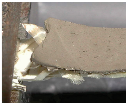
Figure 10. Cracked constant load UV specimen. Break at jaws in upper green layer only on warp yarn. Note "flat" weft yarn.
