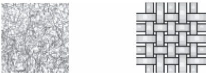
(a) Needle punched nonwoven. (b) Slit-film woven.
