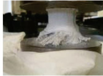
Photo 1. Typical aspect of compression fracture for Portland cement filled jacket.
