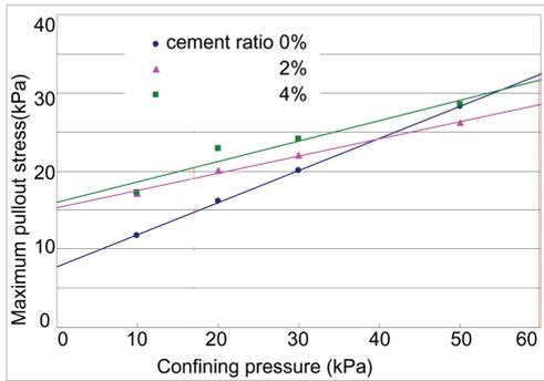
Figure 2. Maximum pullout stress and vertical stress.
