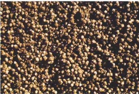
Photo 1. Expanded-beads mixed light-weight soil.
