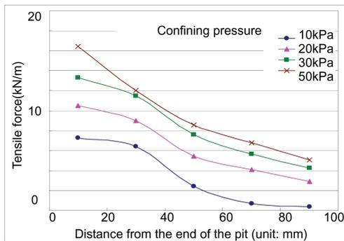
Figure 3. Distribution of the tensile force of the geogrid at the time of the maximum pullout load. (Cement ratio: 0%).
