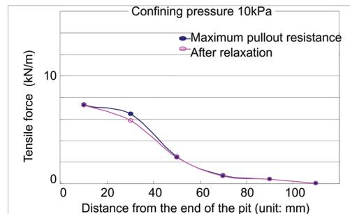
Figure 6. Distribution of the tensile force of the geogrid after relaxation.
