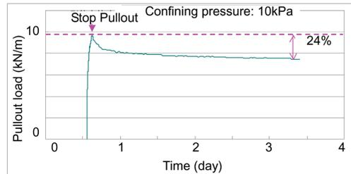
Figure 5. Decline of the pullout load of geogrid in Toyoura sand.
