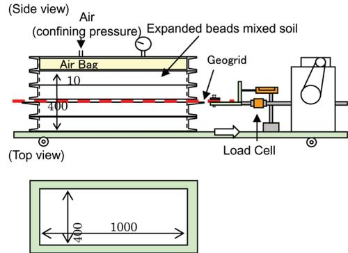
Figure 1. Outline of test facility. (unit: mm)
