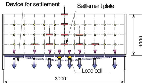
Figure 7. Outline of Test Facility (unit: mm).
