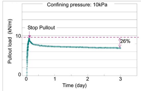
Figure 4. Decline of the pullout load. (Cement ratio: 0%).
