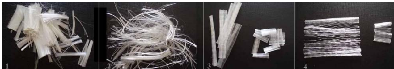
Figure 1. Fibres: 1 – polyester staple fibres, 24 mm; 2 – polyester staple fibres, 70 mm; 3 – polypropylene fibrillated fibres, 24 mm; 4 – polypropylene fibrillated fibres, 70 mm
