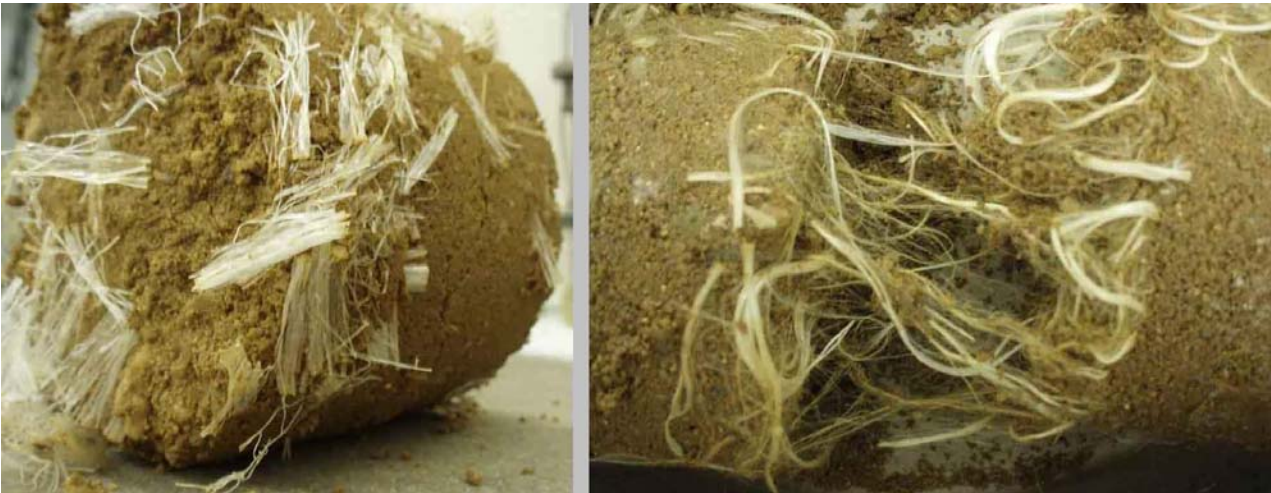
Figure 6. Examples of sandy specimens with short polypropylene fibrillated fibres and long polyester staple fibres
