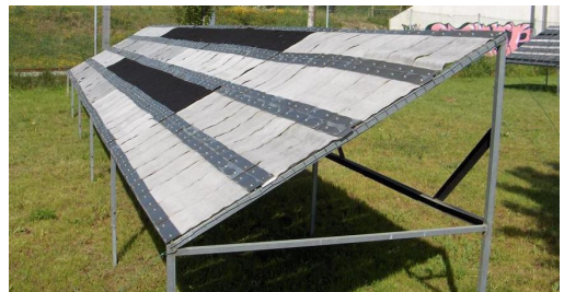
Figure 1. GTXs exposed to natural weathering
