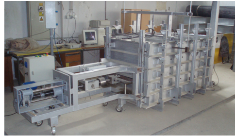
Figure 1. Large pull-out apparatus of GFOS type.
