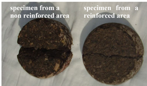
Figure 9. Specimens from areas with (right) and without (left) reinforcement.
