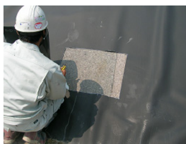
Fig.3 Sampling of geomembranes
