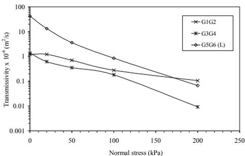
Fig. 6. Variation of transmissivity with type of geocomposites
