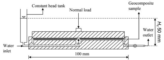
Fig 2. Schematic of transmissivity set-up for geocomposites
