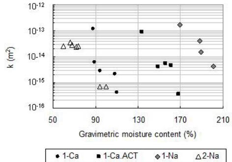
Figure 2. Permeability to gas versus moisture content.
