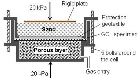
Figure 1. Transient flow permeameter.
