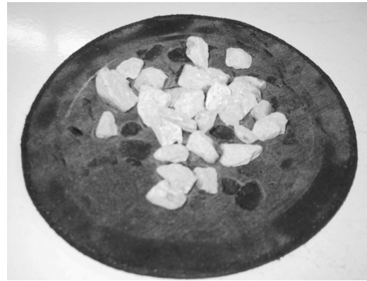
Figure 5. Bituminous geomembrane specimen after the gravel puncturing test.
