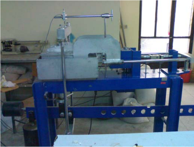
Figure 1. Large direct shear apparatus
