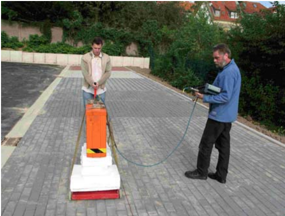
Figure 7. Georadar measurement by the company GBM Wiebe
