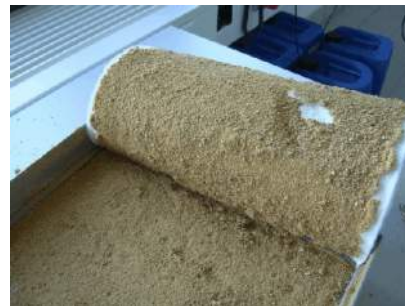
Figure 9. Swelling nonwoven with stuck sand after the test
