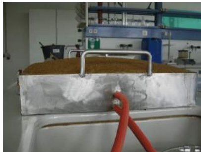
Figure 8. Swelling nonwoven between two sandlayers with enhancement
