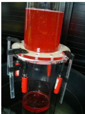
Figure 4. Failed Cylinder test after rust exposure
