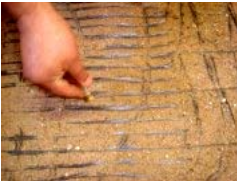
Figure 14. Exhumation of geogrid in a pullout test of geogrid buried in sand
