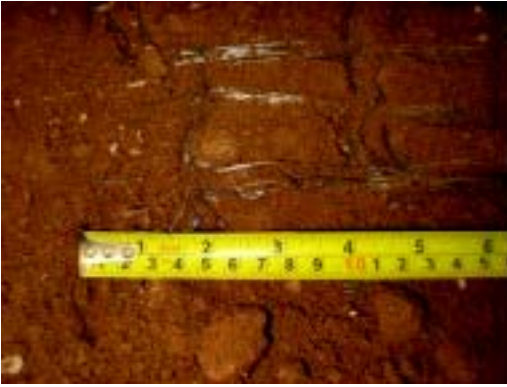
Figure 17. Exhumation of the geogrid used in pullout test of a geogrid buried in RCDW
