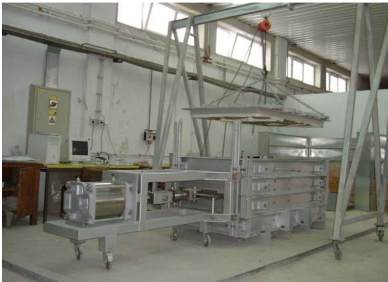
Figure 3. Large pull-out apparatus of GFOS type.
