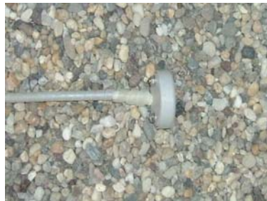
Figure 6. Accelerometer positioning in pullout box.
