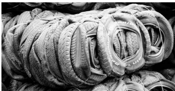
Figure 4. Completed tyre bales.
