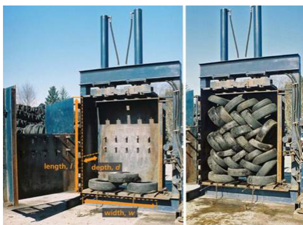
Figure 2. Filling a typical tyre baler using (left) capping tyres to form the bale base; (right) a herring-bone pattern for the body of the bale.
