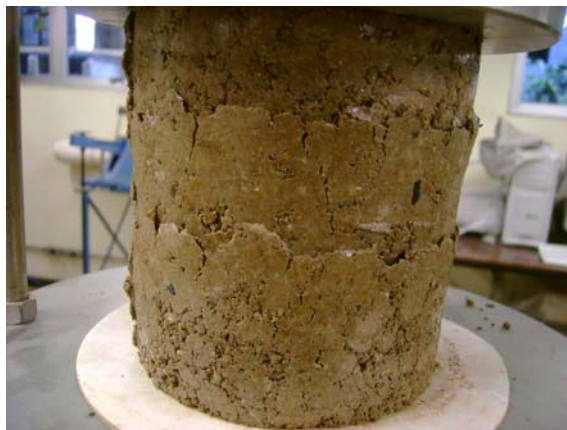
Picture 3. Collapsed sample with woven geotextile incorporation.
