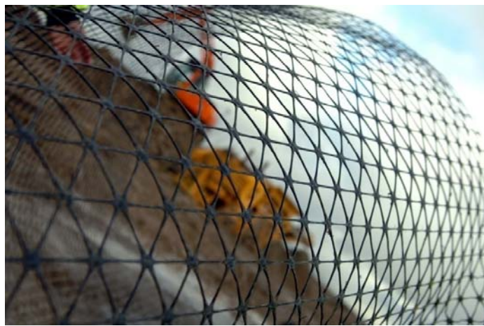
Figure 6: A geogrid with three equilateral rib directions
