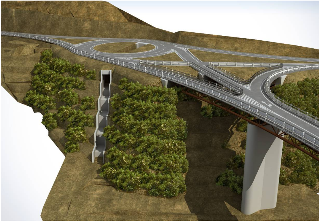
Fig. 1 - Rendering of the Northern round-about, showing the vegetated reinforced soil wall, the Rio Teco channel and the viaduct, whose 3 abutments rest on top of the reinforced soil structure
