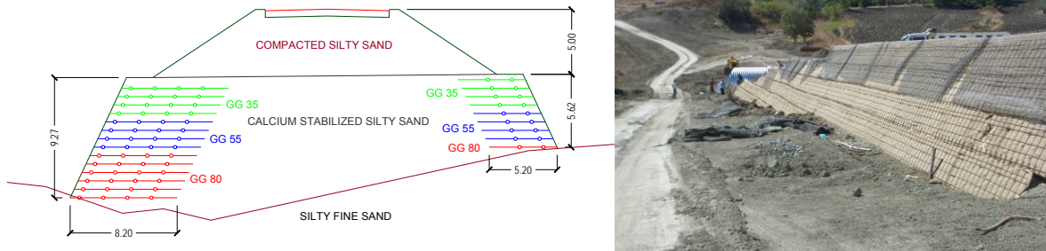
Fig. 12 – Design cross-section and picture of the Bradanica highway embankments during construction
