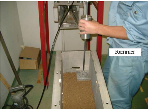
Photo 2. Soil compaction by rammer.
