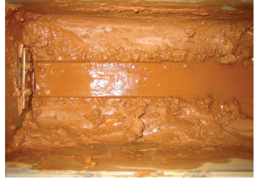
Photo 3. Condition of strip around clay after pullout test (Jiseiji clay).
