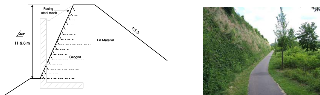
Figure 6. Cross section and picture after full vegetation
